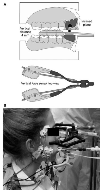
Fig. 1. (A) Schematic representation of the intraoral jaw-positioning device. (B) Participant equipped with all the measurement systems used in the study.
